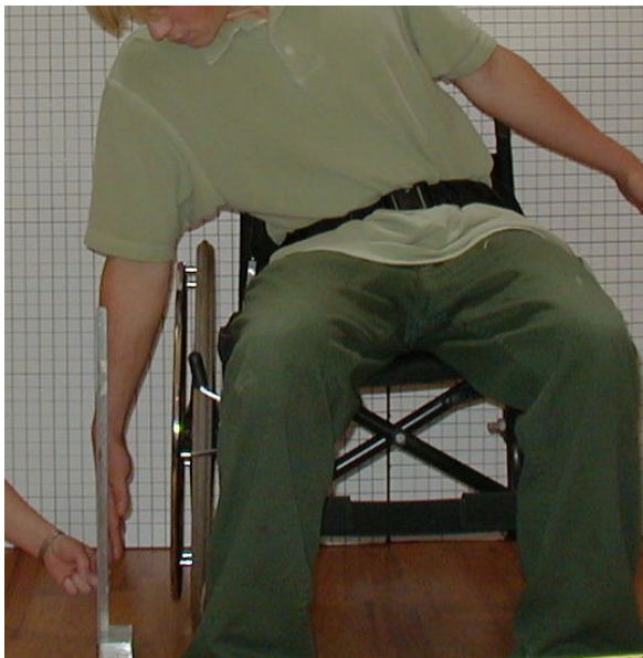
Figure 12. Steel rod setup used to measure downward lean.
