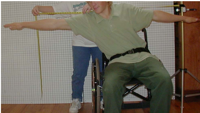
Figure 10. Tripod setup used to measure lateral lean.
