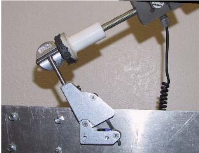
Figure 3. Resistance Force test to 30 degrees
