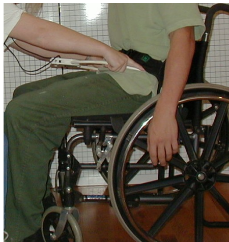
Figure 6. The PALM was used to measure pelvic obliquity.
