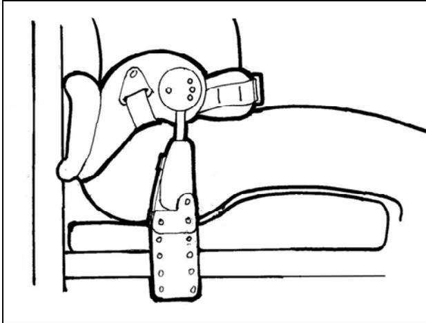
**Figure 1. HipGrip Pelvic Stabilization Device (side view).**
