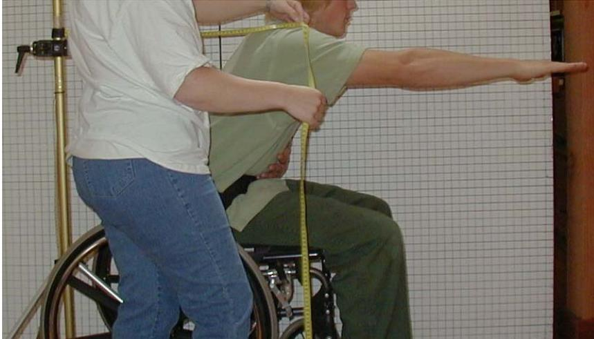
**Figure 8. Tripod setup used to measure forward lean.**
