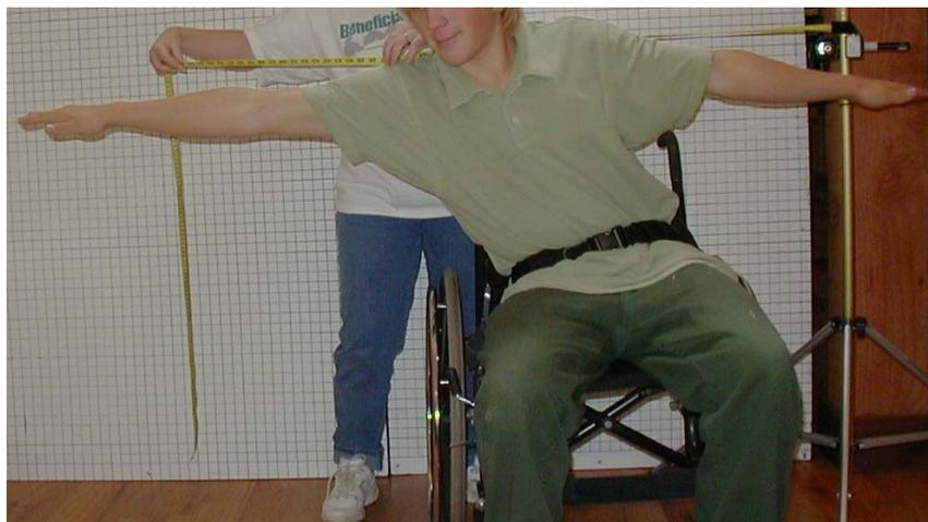
**Figure 10. Tripod setup used to measure lateral lean.**
