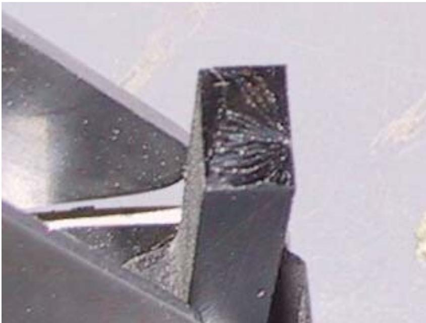
**Figure 3. Broken 2-bump band**
