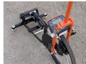
grade, and cross slope on a variety of surfaces, while reducing the number of times an assessor needs to squat or kneel. Developed as a tool to use
