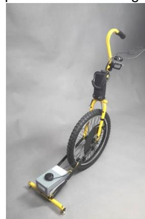
hardware (see UTAP & HETAP Workshops). A fully digital HETAP 3 tilt sensor box with improved accuracy and settling time is available on HETAP 3 carts & rolla-wheels. The cart design boasts a stronger 1.0-inch frame, with solid "no-flat" tires and upholstery that provides improved storage and functionality. Contact us for
