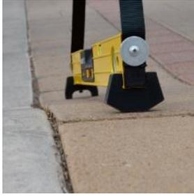
The SmartTool™ offers objective and detailed slope measurements in degrees, percent slope, and pitch to 0.1 degree of resolution and accuracy.
