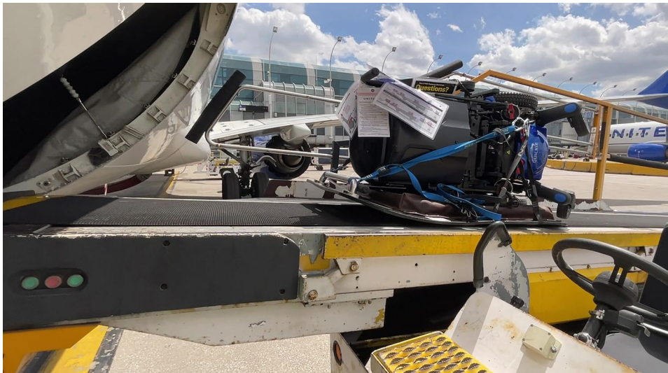
Tipped PWC-PTP package ascending belt loader
