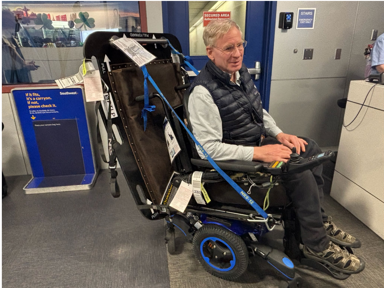
Top and bottom straps hold the PTP against the rear side of the powered wheelchair
