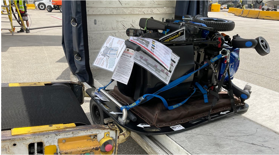
Tipped PWC-PTP package ready to be transferred from baggage trolley to belt loader
