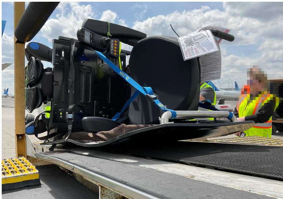
The front and sides of the PTP flex upwards
