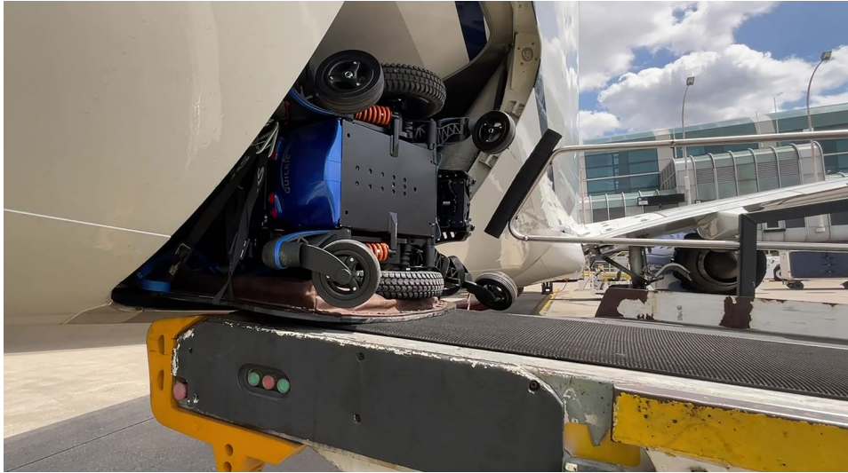
Belt loader pushes PWC-PTP package into a Boeing 737 cargo hold
