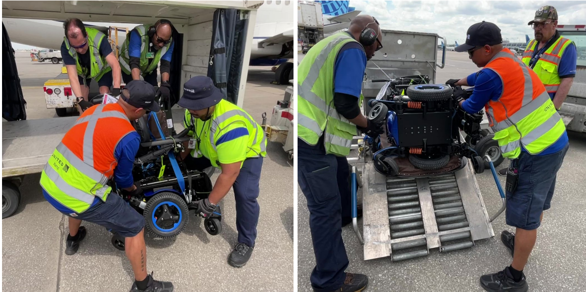
Manually lowering the PWC-PTP package to the ground from a baggage trolley and a KCI wheelchair trailer lift
