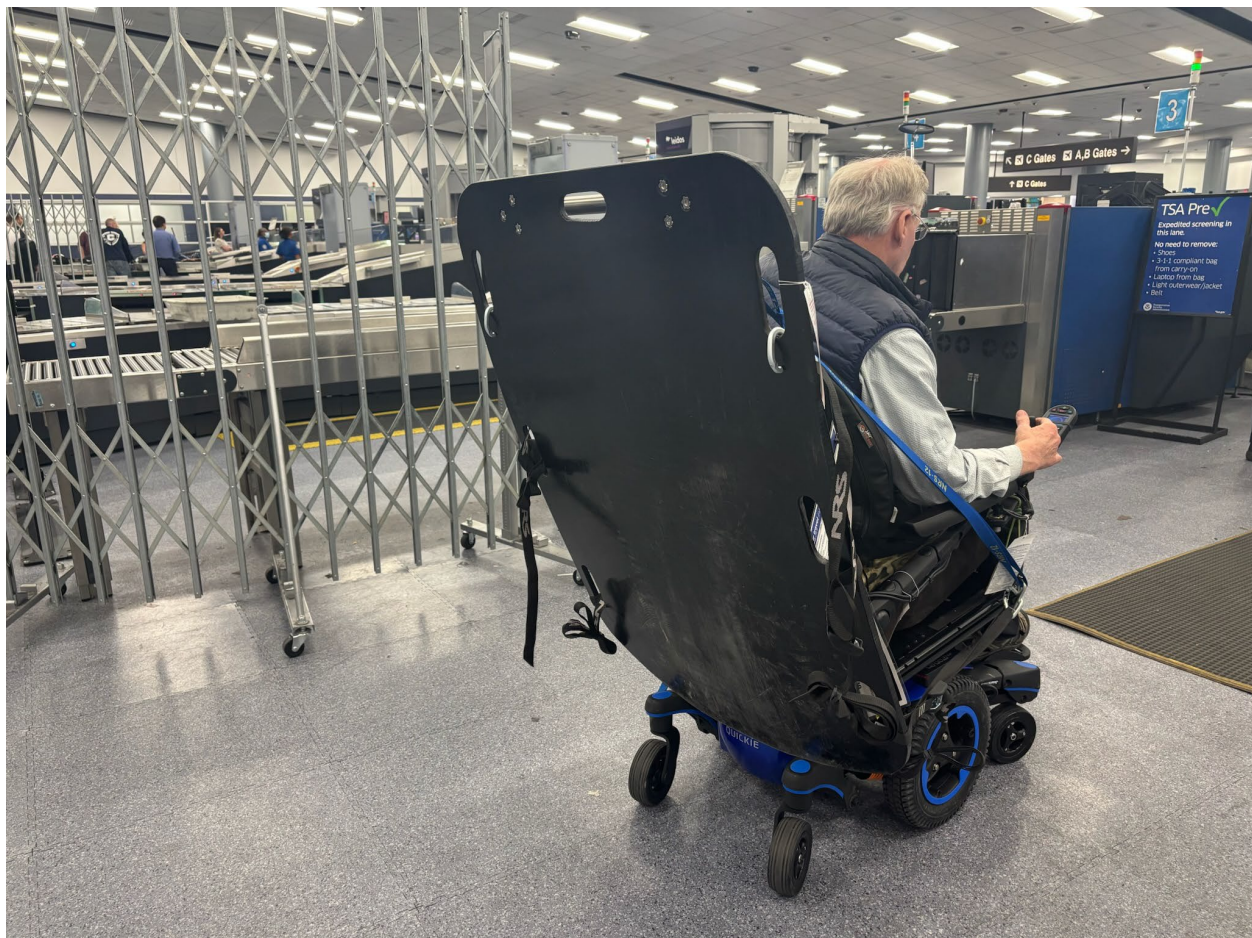
The PTP rests upright on the rear casters of a powered wheelchair
