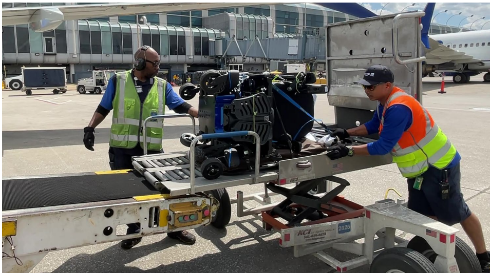
Using a KCI wheelchair trailer lift to transfer the PWC-PTP package
