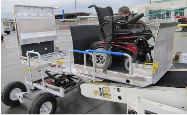
Example of a KCI powered wheelchair trailer lift barge being transferred onto belt loader
